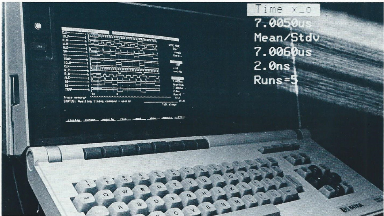
Enhancements to the HP 64600S logic analyzer add new postprocessing functions that let you perform detailed analysis and automated statistical computations of collected timing data in microprocessor-based systems.
