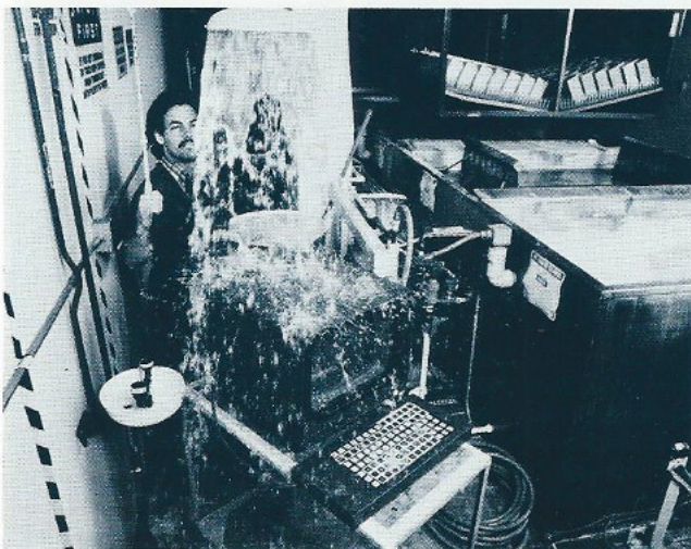
The HP 3092A and 3093A Industrial Display Terminals can actually be cleaned this way. They meet IEC Standard 529, Level 55.
